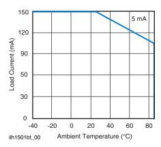
Fig. 1 - Maximum Load Current vs. Ambient Temperature
