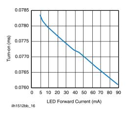
Fig. 16 - Form B Typical Turn-On vs. LED Forward Current
