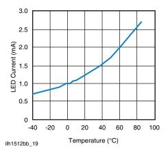
Fig. 19 - Form A Typical I<sub>F</sub> for Switch Operation vs. Temperature
