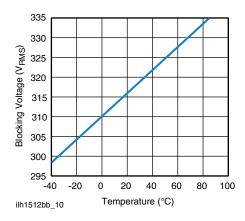
Fig. 10 - Form B Typical Blocking Voltage vs. Temperature
