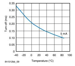
Fig. 9 - Form A Typical Turn-Off vs. Temperature
