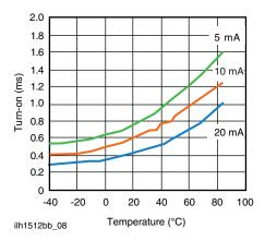
Fig. 8 - Form A Typical Turn-On vs. Temperature
