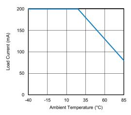
Fig. 1 - Maximum Load Current vs. Ambient Temperature
