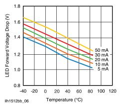
Fig. 6 - Typical LED Forward Voltage Drop vs. Temperature
