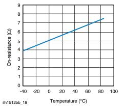
Fig. 18 - Form B Typical On-Resistance vs. Temperature
