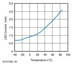
Fig. 20 - Form A Typical I<sub>F</sub> for Switch Dropout vs. Temperature
