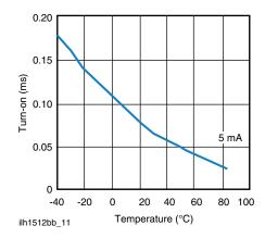
Fig. 11 - Form B Typical Turn-On vs. Temperature
