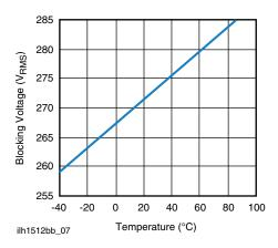
Fig. 7 - Form A Typical Blocking Voltage vs. Temperature
