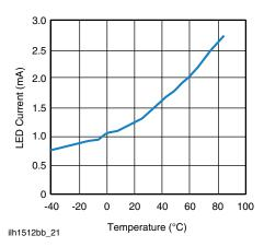
Fig. 21 - Form B Typical I<sub>F</sub> for Switch Operation vs. Temperature
