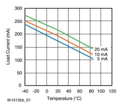
Fig. 2 - Form A Typical Load Current vs. Temperature
