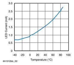
Fig. 22 - Form B Typical I<sub>F</sub> for Switch Dropout vs. Temperature
