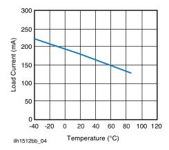
Fig. 5 - Form B Typical Load Current vs. Temperature
