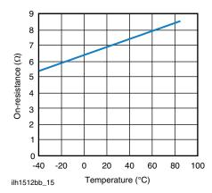
Fig. 15 - Form A Typical On-Resistance vs. Temperature
