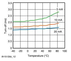
Fig. 12 - Form B Typical Turn-Off vs. Temperature
