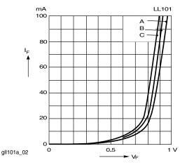
Fig. 2 - Typ.  $I_F$  of Combination Schottky Barrier and PN Junction Guard Ring
