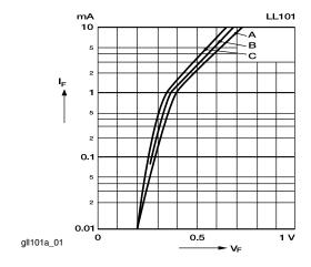
Fig. 1 - Typ. I<sub>F</sub> vs. V<sub>F</sub> for Primary Conduction through the Schottky Barrier
