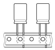
Fig. 3 - Form TFA: taped in box (ammopack)
