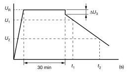
Fig. 4 - Voltage Diagram for Capacitance Measurement
