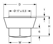
Fig. 7 - Synthetic cap nut; see Table 2 for dimensions D, H and W
