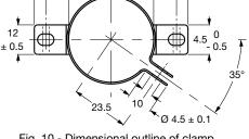
Fig. 10 - Dimensional outline of clamp for case Ø D = 35 mm
