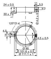
Fig. 5 - Dimensional outline of clamp for case  $\emptyset$  D = 90 mm
