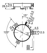
Fig. 4 - Dimensional outline of clamp for case  $\emptyset$  D = 76 mm
