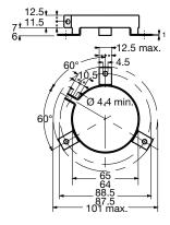
Fig. 3 - Dimensional outline of clamp for case  $\emptyset$  D = 65 mm
