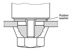
Fig. 6 - Insulated mounting
