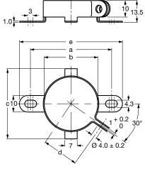
Fig. 9 - Dimensional outline of clamp for case  $\emptyset$  D = 25 mm, 30 mm and 40 mm
