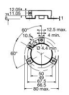
Fig. 2 - Dimensional outline of clamp for case Ø D = 50 mm
