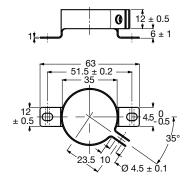
Fig. 1 - Dimensional outline of clamp for case  $\emptyset$  D = 35 mm
