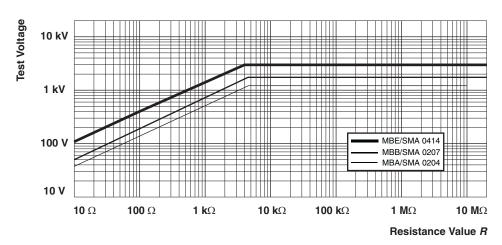
Pulse load rating in accordance with IEC 60115-1, 4.27; 10  $\mu$ s/700  $\mu$ s; 10 pulses at 1 minute intervals; for permissible resistance change (0.5 % R + 0.05  $\Omega$ )
