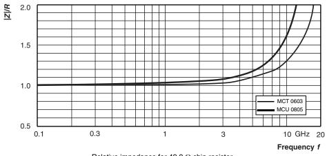
Relative impedance for 49.9  $\Omega$  chip resistor
