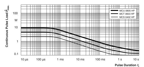
Maximum pulse load, continuous pulses; applicable if  $\overline{P} \leq P$  ( $\mathcal{G}_{amb}$ ) and  $\hat{U} \leq \hat{U}_{max}$ ; for permissible resistance change  $\pm$  (0.5 % R + 0.05  $\Omega$ )
