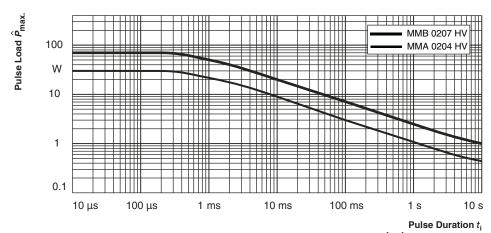
$\label{eq:max} \textbf{Maximum pulse load, single pulse; applicable if $\bar{P} \to 0$ and $n \le 1000$ and $\hat{U} \le \hat{U}_{max}$;} \\ \textbf{Single Pulse} \qquad \qquad \text{for permissible resistance change equivalent to 8000 h operation in power operation model}$
