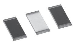
Vishay's proven precision thin film wraparound resistors will meet your exact requirements. These resistors are ideal for use in oil industry precision applications requiring low noise, long term stability under high temperature, ultra low temperature coefficient of resistance, and low voltage coefficient. The chip resistors are available in any resistance ohmic value in the range specified below.
