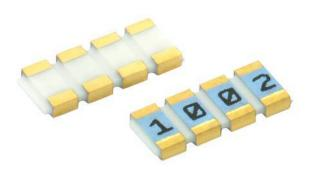
PRAHT arrays can be used in most applications requiring a matched pair (or set) of resistor elements at very high temperature up to 230 °C. The networks provide 2 ppm/°C TCR tracking, a ratio tolerance as tight as 0.05 % and outstanding stability.
