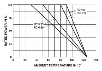
For resistors mounted onto heatsink and thermal resistance
