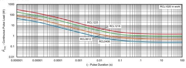
Maximum pulse load, continuous pulses; applicable if  $\bar{P} \leq P\left(\mathcal{G}_{amb}\right)$  and  $\hat{U} \leq \hat{U}_{max}$ ; for permissible resistance change equivalent to 8000 h operation
