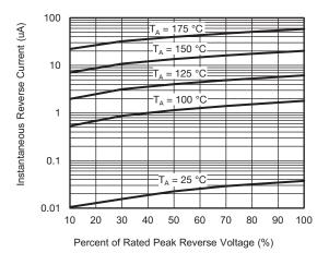
Fig. 4 - Typical Reverse Leakage Characteristics
