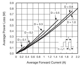
Fig. 2 - Average Power Loss Characteristics
