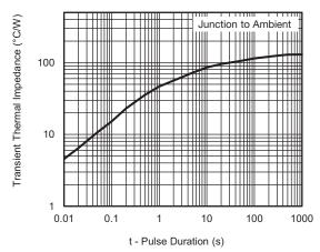
Fig. 6 - Typical Transient Thermal Impedance
