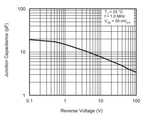
Fig. 5 - Typical Junction Capacitance
