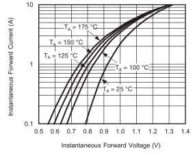
Fig. 3 - Typical Instantaneous Forward Characteristics
