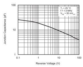
Fig. 5 - Typical Junction Capacitance
