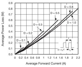
Fig. 2 - Average Power Loss Characteristics
