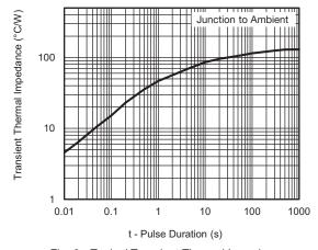
Fig. 6 - Typical Transient Thermal Impedance
