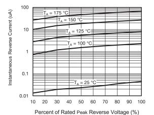
Fig. 4 - Typical Reverse Leakage Characteristics
