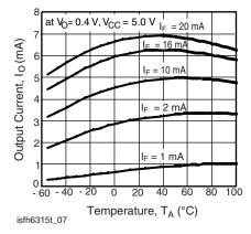
Fig. 6 - Output Current vs. Temperature
