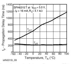
Fig. 8 - Propagation Delay vs. Temperature SFH6315T
