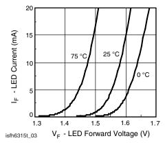
Fig. 3 - LED Forward Current vs. Forward Voltage
