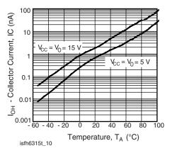
Fig. 9 - Logic High Output Current vs.Temperature
