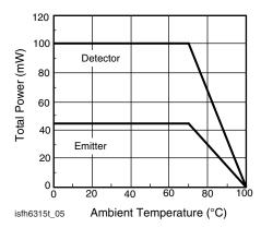
Fig. 5 - Permissible Power Dissipation vs. Temperature
