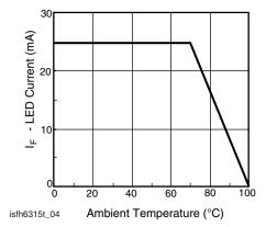
Fig. 4 - Permissible Forward LED Current vs. Temperature
