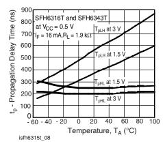
Fig. 7 - Propagation Delay vs. Temperature SFH6316T and SFH6343T
