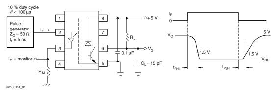
Fig. 1 - Test Circuit for Switching Times
