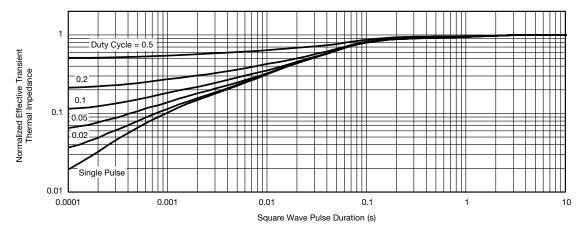
Normalized Thermal Transient Impedance, Junction-to-Foot
