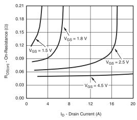
On-Resistance vs. Drain Current
