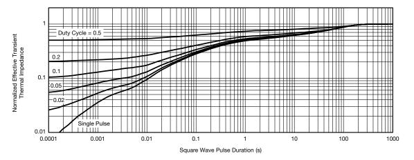
Normalized Thermal Transient Impedance, Junction-to-Ambient
