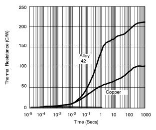
FIGURE 5. Leadframe Comparison on Alloy 42 1-inch<sup>2</sup> PCB
