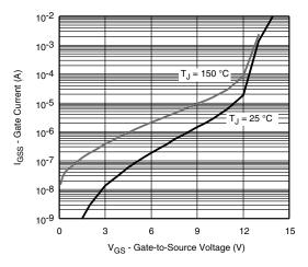
Gate Current vs. Gate-Source Voltage
