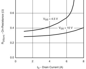
**On-Resistance vs. Drain Current and Gate Voltage**
