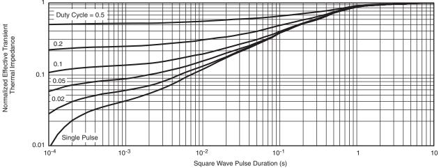
Normalized Thermal Transient Impedance, Junction-to-Foot
