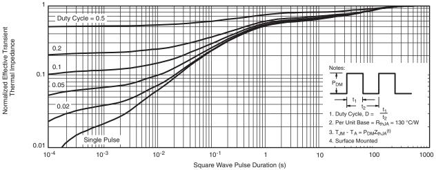
Normalized Thermal Transient Impedance, Junction-to-Ambient
