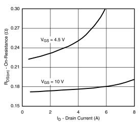
On-Resistance vs. Drain Current and Gate Voltage
