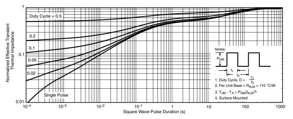
Normalized Thermal Transient Impedance, Junction-to-Ambient
