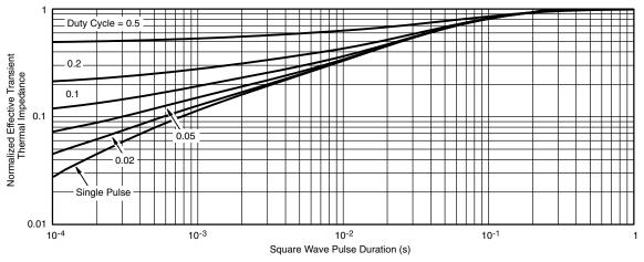
Normalized Thermal Transient Impedance, Junction-to-Foot
