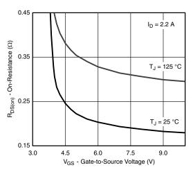
On-Resistance vs. Gate-to-Source Voltage
