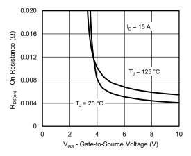
On-Resistance vs. Gate-to-Source Voltage
