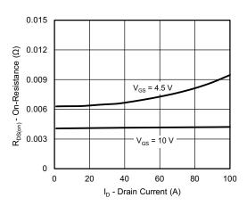
On-Resistance vs. Drain Current and Gate Voltage
