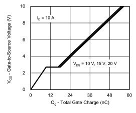
Gate Charge On-Resistance vs. Junction Temperature
