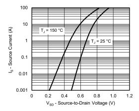
Source-Drain Diode Forward Voltage
