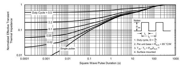
Normalized Thermal Transient Impedance, Junction-to-Ambient
