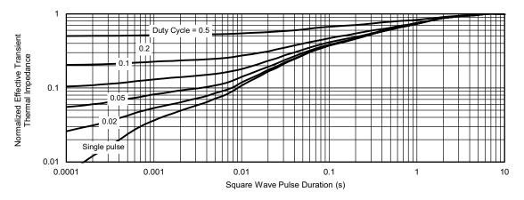
Normalized Thermal Transient Impedance, Junction-to-Case
