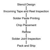
FIGURE 5. SMT Assembly Process Flow
