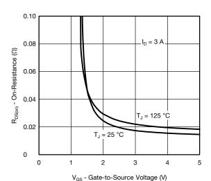
On-Resistance vs. Gate-to-Source Voltage
