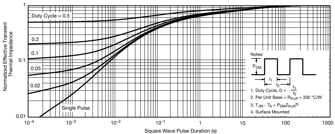
Normalized Thermal Transient Impedance, Junction-to-Ambient (On 1" x 1" FR4 Board with Minimum Copper)
