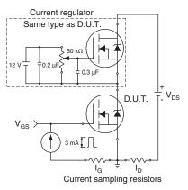
Fig. 18 - Gate Charge Test Circuit
