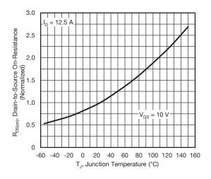
Fig. 4 - Normalized On-Resistance vs. Temperature
