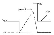
Fig. 16 - Unclamped Inductive Waveforms
