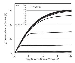
Fig. 1 - Typical Output Characteristics
