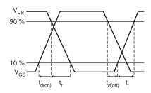
Fig. 14 - Switching Time Waveforms
