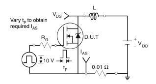
Fig. 15 - Unclamped Inductive Test Circuit
