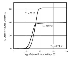
Fig. 3 - Typical Transfer Characteristics
