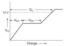
Fig. 17 - Basic Gate Charge Waveform
