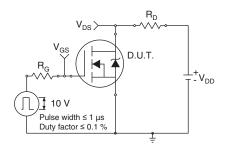
Fig. 13 - Switching Time Test Circuit
