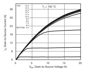
Fig. 2 - Typical Output Characteristics
