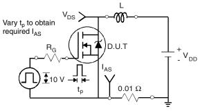
Fig. 15 - Unclamped Inductive Test Circuit
