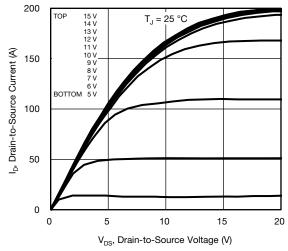
Fig. 1 - Typical Output Characteristics
