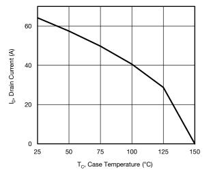
Fig. 10 - Maximum Drain Current vs. Case Temperature
