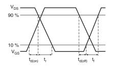
Fig. 14 - Switching Time Waveforms
