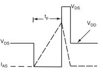
Fig. 16 - Unclamped Inductive Waveforms
