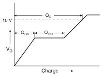
Fig. 17 - Basic Gate Charge Waveform
