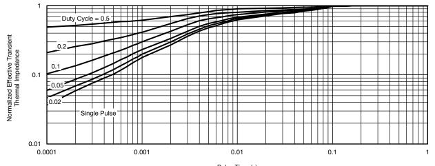
Pulse Time (s) Fig. 12 - Normalized Thermal Transient Impedance, Junction-to-Case
