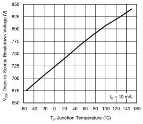
Fig. 11 - Temperature vs. Drain-to-Source Voltage
