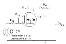
Fig. 13 - Switching Time Test Circuit
