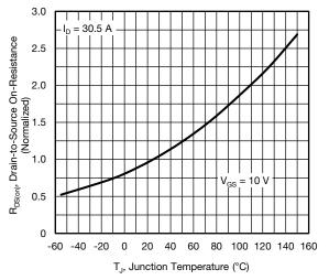
Fig. 4 - Normalized On-Resistance vs. Temperature
