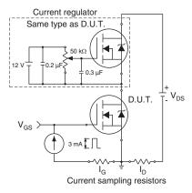
Fig. 18 - Gate Charge Test Circuit
