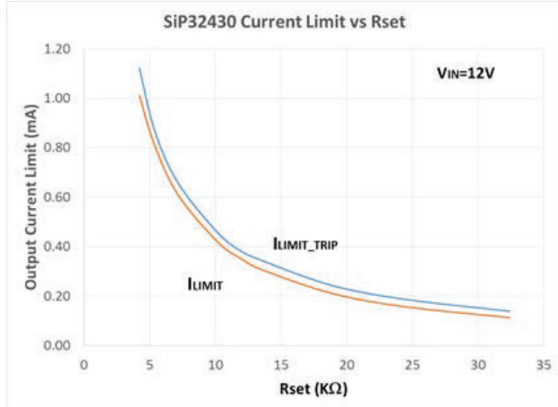
Fig. 47 - Current Limit vs. R SET
