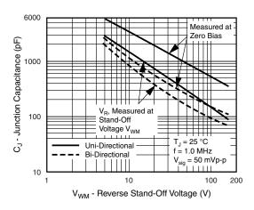
Fig. 4 - Typical Junction Capacitance
