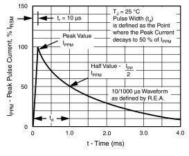
Fig. 3 - Pulse Waveform
