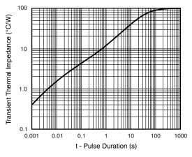
Fig. 5 - Typical Transient Thermal Impedance
