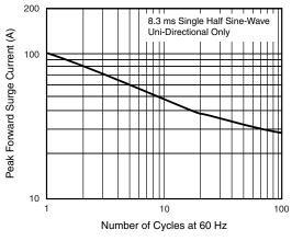
Fig. 6 - Maximum Non-Repetitive Forward Surge Current
