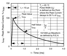
Fig. 3 - Pulse Waveform
