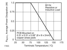
Fig. 1 - Maximum Continuous Power Dissipation
