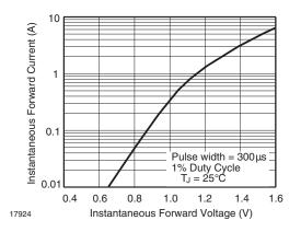
Fig. 4 - Typical Instantaneous Forward Characteristics for SML4763
