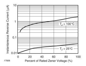
Fig. 5 - Typical Reverse Characteristics
