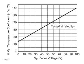
Fig. 3 - Typical Temperature Coefficients
