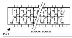
TTL dual-line terminator; pulse squaring, 14 or 18 pairs of resistors
