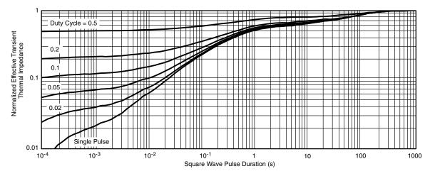
Normalized Thermal Transient Impedance, Junction-to-Ambient
