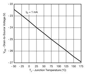
**Drain Source Breakdown vs. Junction Temperature**
