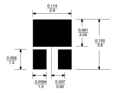
FIGURE 1. Footprint With Copper Spreading
