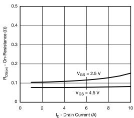
On-Resistance vs. Drain Current
