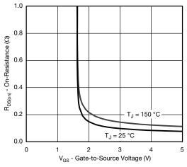
On-Resistance vs. Gate-to-Source Voltage
