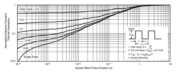
Normalized Thermal Transient Impedance, Junction-to-Foot
