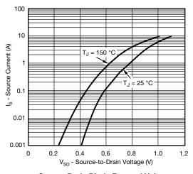
Source-Drain Diode Forward Voltage
