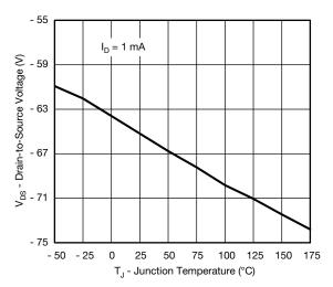
Drain Source Breakdown vs. Junction Temperature
