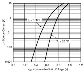
Source-Drain Diode Forward Voltage
