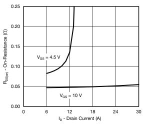
On-Resistance vs. Drain Current
