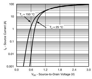
**Source Drain Diode Forward Voltage**
