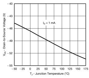
Drain Source Breakdown vs. Junction Temperature
