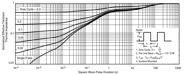
Normalized Thermal Transient Impedance, Junction-to-Ambient
