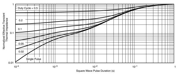
Normalized Thermal Transient Impedance, Junction-to-Foot
