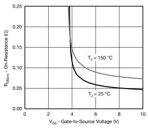
On-Resistance vs. Gate-to-Source Voltage
