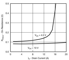
**On-Resistance vs. Drain Current and Gate Voltage**
