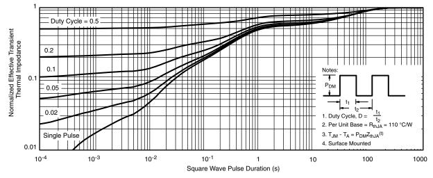
Normalized Thermal Transient Impedance, Junction-to-Ambient
