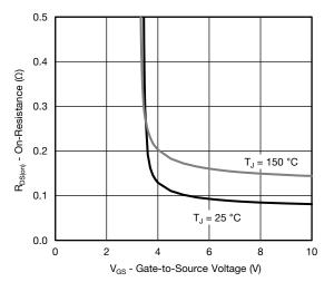
**On-Resistance vs. Gate-to-Source Voltage**
