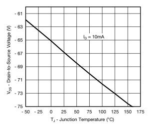
Drain-to-Source Voltage vs. Junction Temperature
