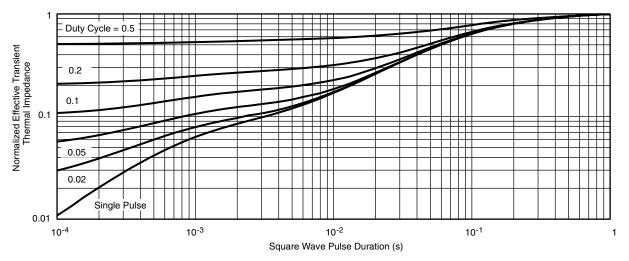
Normalized Thermal Transient Impedance, Junction-to-Foot
