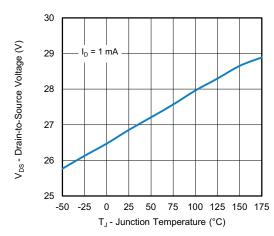
Drain Source Breakdown vs. Junction Temperature
