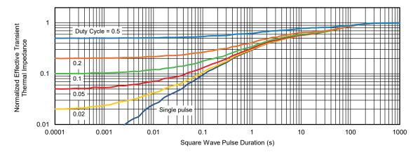
Normalized Thermal Transient Impedance, Junction-to-Foot
