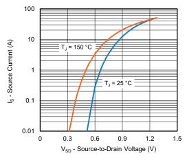
**Source Drain Diode Forward Voltage**
