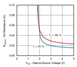
On-Resistance vs. Gate-to-Source Voltage
