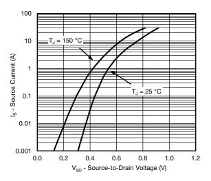
Source Drain Diode Forward Voltage
