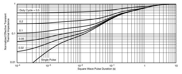
Normalized Thermal Transient Impedance, Junction-to-Foot
