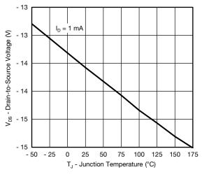
Breakdown Voltage vs. Junction Temperature
