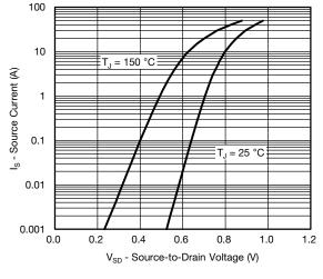
**Source Drain Diode Forward Voltage**
