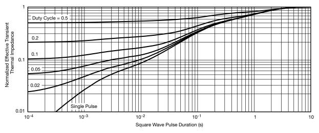
Normalized Thermal Transient Impedance, Junction-to-Ambient
