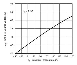
Drain Source Breakdown vs. Junction Temperature
