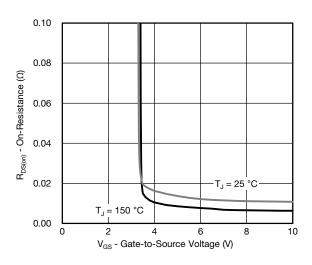
On-Resistance vs. Gate-to-Source Voltage
