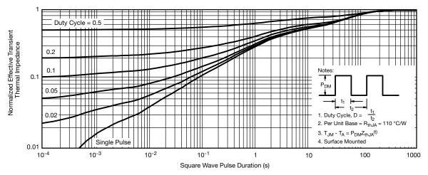
Normalized Thermal Transient Impedance, Junction-to-Ambient
