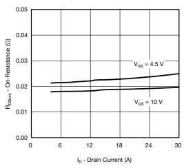
On-Resistance vs. Drain Current
