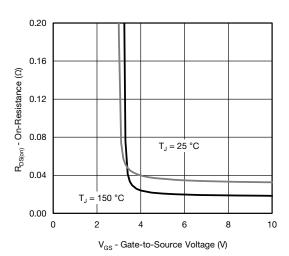
On-Resistance vs. Gate-to-Source Voltage
