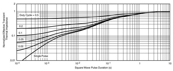
Normalized Thermal Transient Impedance, Junction-to-Foot
