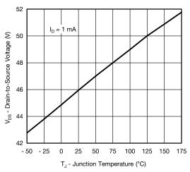
**Drain Source Breakdown vs. Junction Temperature**
