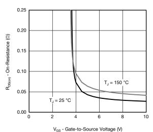
On-Resistance vs. Gate-to-Source Voltage
