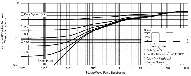
Normalized Thermal Transient Impedance, Junction-to-Ambient
