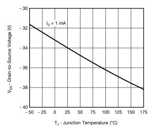
Drain Source Breakdown vs. Junction Temperature
