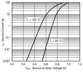
**Source Drain Diode Forward Voltage**
