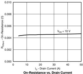
On-Resistance vs. Drain Current
