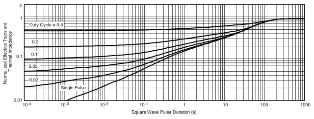
Normalized Thermal Transient Impedance, Junction-to-Ambient
