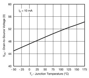
Drain Source Breakdown vs. Junction Temperature
