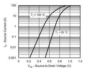
Source Drain Diode Forward Voltage
