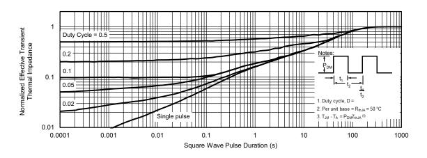
Normalized Thermal Transient Impedance, Junction-to-Ambient
