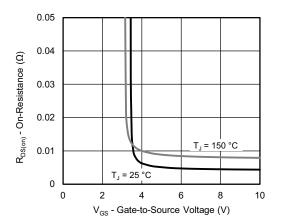
On-Resistance vs. Gate-to-Source Voltage
