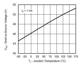
Drain Source Breakdown vs. Junction Temperature
