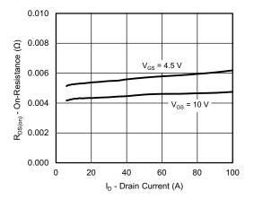
**On-Resistance vs. Drain Current**
