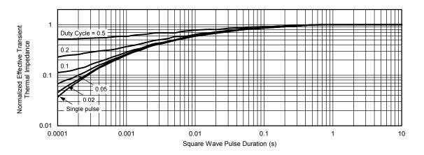
Normalized Thermal Transient Impedance, Junction-to-Case
