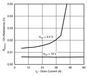
On-Resistance vs. Drain Current
