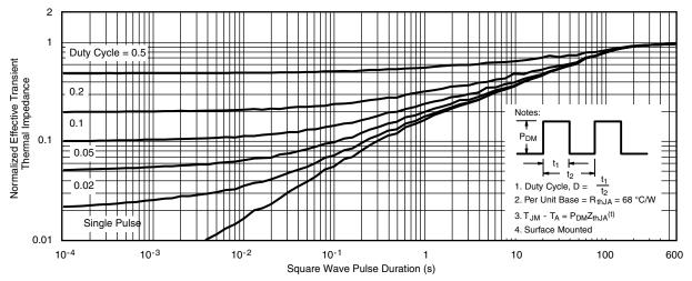
Normalized Thermal Transient Impedance, Junction-to-Ambient
