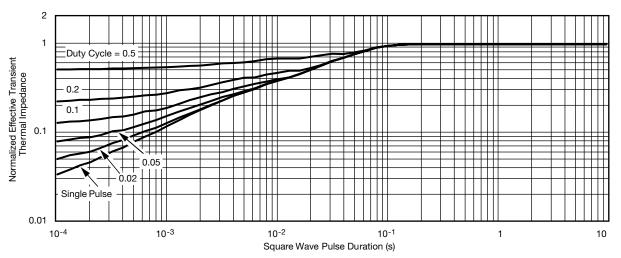
Normalized Thermal Transient Impedance, Junction-to-Case
