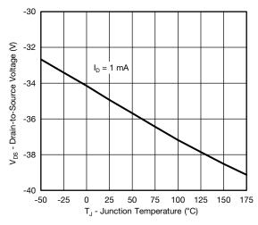
**Drain Source Breakdown vs. Junction Temperature**
