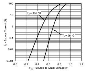
**Source Drain Diode Forward Voltage**
