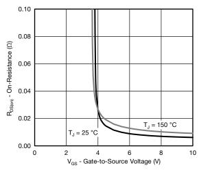
On-Resistance vs. Gate-to-Source Voltage
