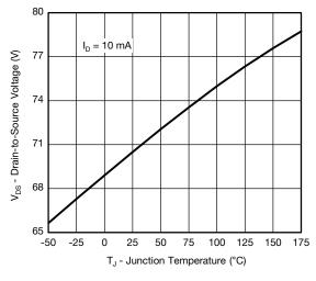
Drain Source Breakdown vs. Junction Temperature
