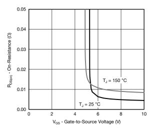
On-Resistance vs. Gate-to-Source Voltage
