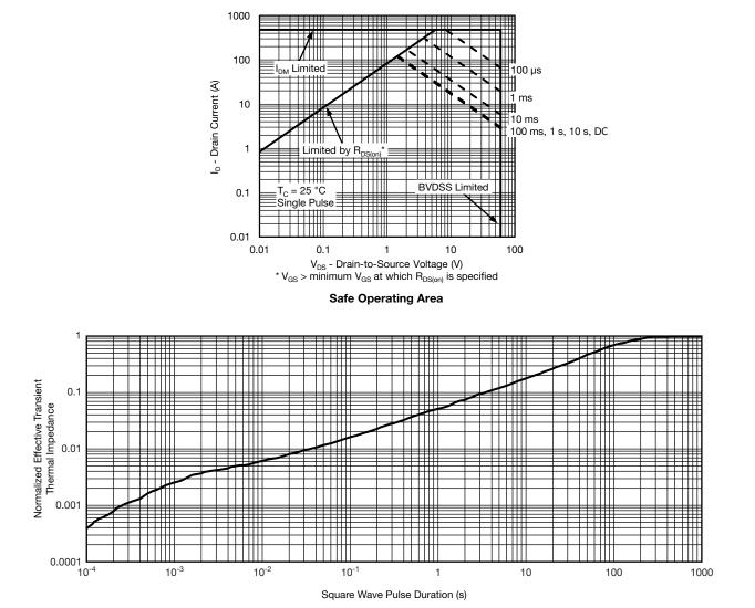
Normalized Thermal Transient Impedance, Junction-to-Ambient
