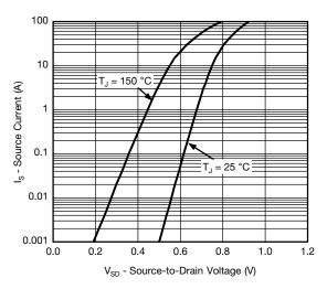
Source Drain Diode Forward Voltage
