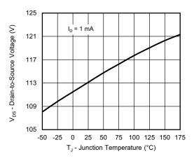
**Drain Source Breakdown vs. Junction Temperature**
