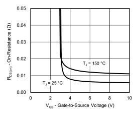
On-Resistance vs. Gate-to-Source Voltage
