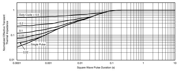
Normalized Thermal Transient Impedance, Junction-to-Case
