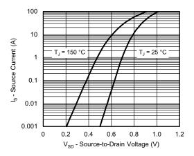
**Source Drain Diode Forward Voltage**
