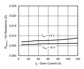
On-Resistance vs. Drain Current
