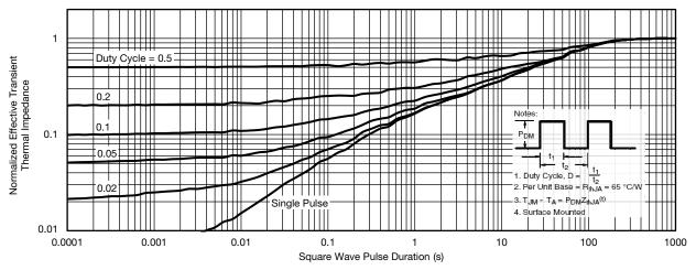
Normalized Thermal Transient Impedance, Junction-to-Ambient
