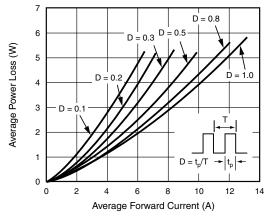
Fig. 2 - Forward Power Loss Characteristics
