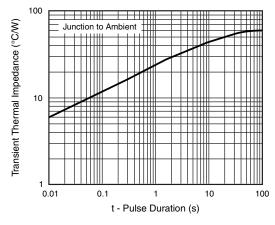
Fig. 6 - Typical Transient Thermal Impedance
