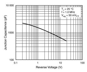
Fig. 5 - Typical Junction Capacitance
