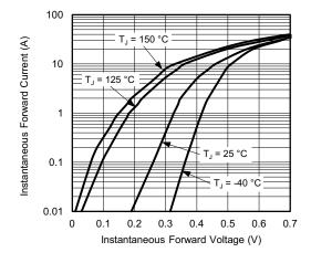
Fig. 3 - Typical Instantaneous Forward Characteristics
