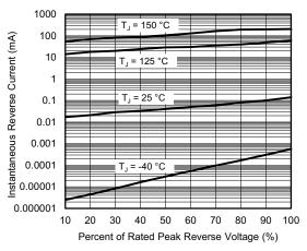
Fig. 4 - Typical Reverse Leakage Characteristics
