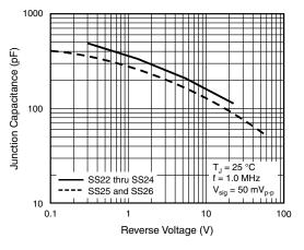
Fig. 5 - Typical Junction Capacitance
