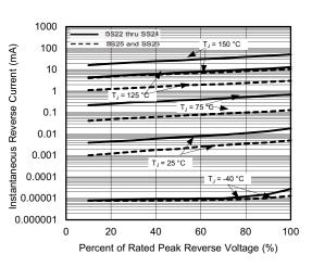
Fig. 4 - Typical Reverse Current Characteristics
