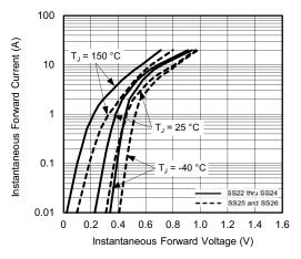
Fig. 3 - Typical Instantaneous Forward Characteristics
