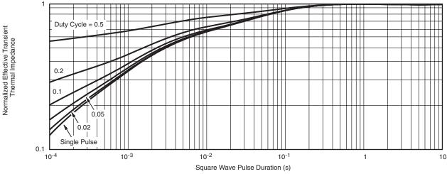
Normalized Thermal Transient Impedance, Junction-to-Case
