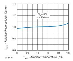
Fig. 2 - Relative Reverse Light Current vs. Ambient Temperature
