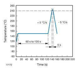
Fig. 7 - Lead Tin (SnPb) Reflow Solder Profile
