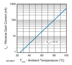
Fig. 1 - Reverse Dark Current vs. Ambient Temperature
