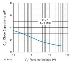
Fig. 4 - Diode Capacitance vs. Reverse Voltage
