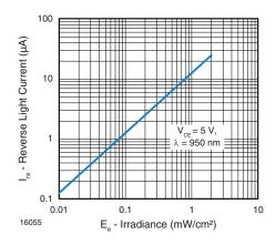
Fig. 3 - Reverse Light Current vs. Irradiance
