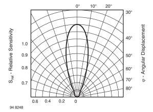
Fig. 8 - Relative Radiant Sensitivity vs. Angular Displacement
