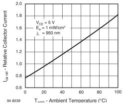
Fig. 3 - Relative Collector Current vs. Ambient Temperature
