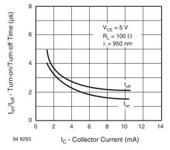
Fig. 6 - Turn-on/Turn-off Time vs. Collector Current
